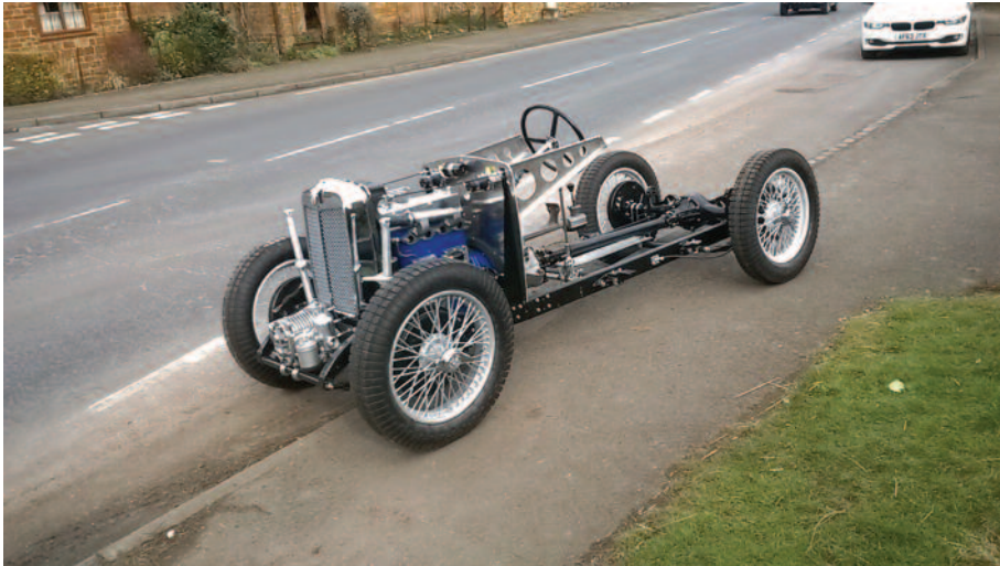
Photo 5: Complete chassis about to be transported to Worksop for the body to be fitted.
